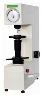
iRock-431M Motorized Rockwell hardness tester adopts the mechanism of automatic loading and unloading of the test force, the test force is regulated by the load-change hand wheel. It can select the dwell time and is very easy to use. Besides setting zero to dial, there is no man-made error. The instrument has high sensitivity and stability.
